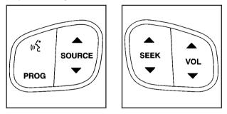
(**C** (OnStar/Voice Recognition): If you vehicle has OnStar<sup>®</sup>, you can press this button to interact with the OnStar<sup>®</sup> system. See the OnStar<sup>®</sup> manual provided with your vehicle for more information.
